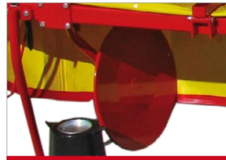
**3** Disc conveyor bolted on top of guard support to avoid wrapping problems.
