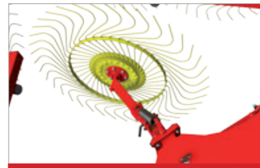
3 Optional hydraulically raised Kicker wheel available for all sizes.
